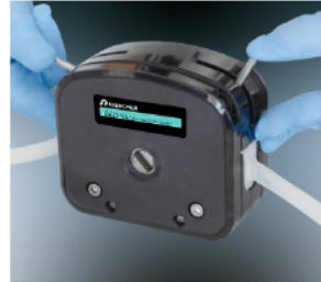
C. Install the upper block, put down the levers to lock the block.
