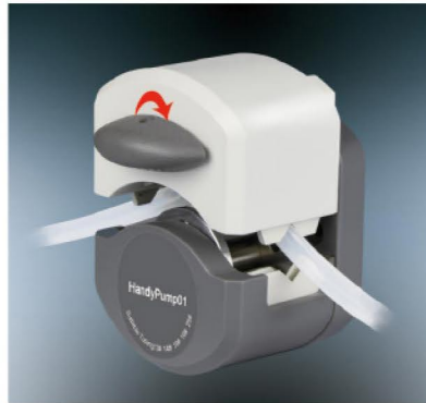
B. Put the tube between rollers and upper block, tighten up the tubing lightly.
